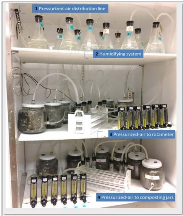
Figure 3. Laboratory apparatus employed to measure the biodegradability of plastic mulches under composting conditions via the ASTM D5338 standardized laboratory test.
